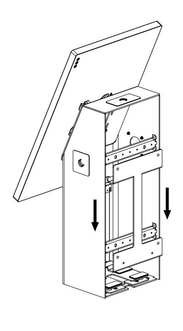
**Step 5:** Remove the printer cover, and attach the module to the wall bracket with the two M5 x 12mm screws.
