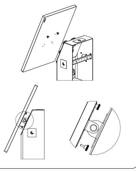
**Step 2:** To adjust the height of the screen, loosen the four screws slightly. Set the VESA mount to the desired height, and tighten the screws securely.
